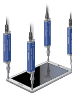
Smartphone flatness measurement
